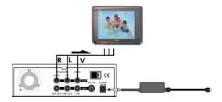
To connect to a SCART input, a three phono (RCA) plug (Left and Right Audio plus Composite Video) to SCART Plug cable will be required.
