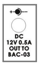
DC 12V 0.5A output to connect BAC-03 Audio converter
