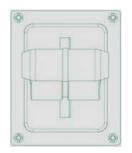
T-bar is for performing effect transitions manually. It can be either all the way up, all the way down, or anywhere in between. To enable the SE-800 T-Bar, the T-Bar on RMC-90 must be at either end of its travel.
