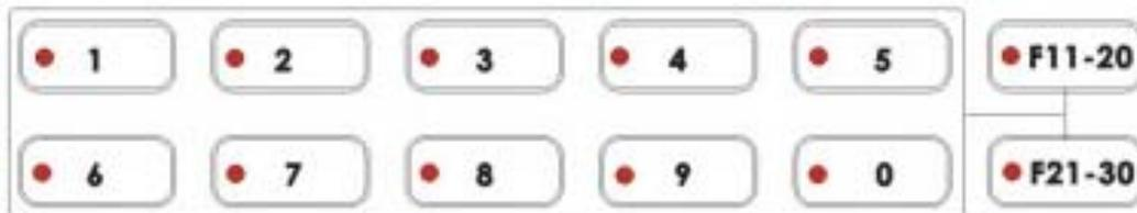
These preset Banks offer 30 memory locations to store transitions or effects that will be executed at the touch of a button. The numbered buttons 1-0 above accesses 10 locations. First pressing the F11-20 button until the LED on it is lit, then pressing one of the single numbered buttons access presets 11-20. Pressing the F21-30 button, then one of the single numbered buttons, accesses presets 21-30.
