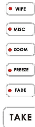
20. Transition selectors: These five selection buttons determine the transition type and allow for the selection of certain effects that are performed on the selected Main Video Input channel. The Take-button executes an auto play. For more information, see **Using Transitions**, page 35 and **Using Effects**, page 41.
