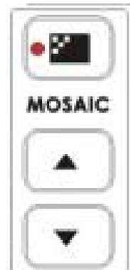
The effect can be applied to the whole image or one of two window sizes, which can be positioned anywhere on the screen, using the Joystick in Position Control Mode. The size of the effect window is represented by numbers 1-2 displayed in the Speed window above the Keypad, and may be changed by pressing the UP and DOWN Arrow buttons beneath the PIP button.
