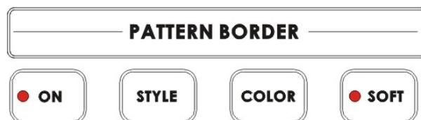
10. Background: when Background is selected in either the Main or Sub Video Source (4, 5.), and the On button is pressed (and the LED is lit), repeated presses of the color button cycle through the 8 possible solid backgrounds. For more information, see **Background**, page 44.
