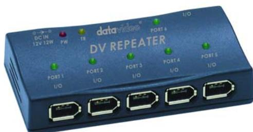
One input to five channels output DV-DA (VP-332)
