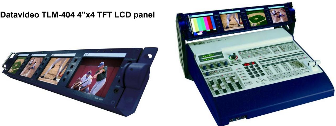
Datavideo TLM-404 is a 4x4" TFT LCD monitors, 2U height design for standard 19" rack mount. NTSC/PAL video format auto recognition with video pass through 75-ohm self-terminated video output connector. The "AUX" input provides options for external format converters such as SDI and DV input converter. The tilt hinges let you tilt the screen +/- 30 degree with contrast, brightness, color and tint (Tint only available for NTSC) controls for a best view quality of display.
