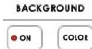
Engage this control by pressing the "ON" button in this section. The LED on the button will blink to indicate that the controls are active. Repeated presses of the "COLOR" button select colors: 1 is black, 8 is white.
